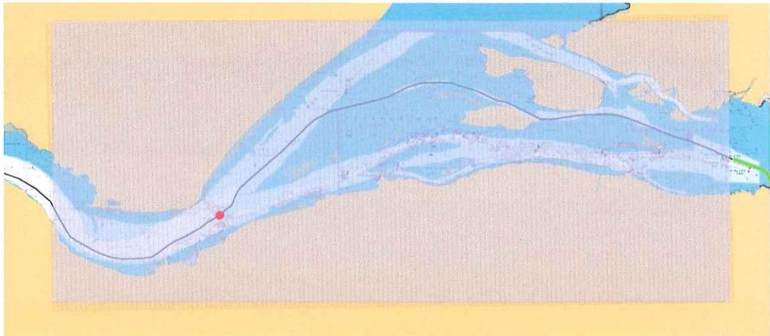
The size of the sample box is determined by the anchor dragging distance. In Intertek's experience, under normal weather conditions, when first deployed, most anchors tend to drag less than 200 feet before engaging (DONG Energy, 2012). Hence the size of a sample box is 200 feet.
